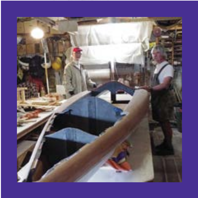
Robertson and Izon fitting the floorboards.
